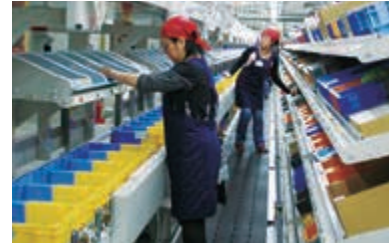
Pick-to-light system – Digital Pick System
