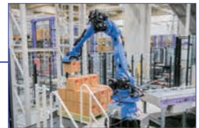
Depalletizing robot Picks cardboard boxes from a pallet retrieved from an AS/RS
