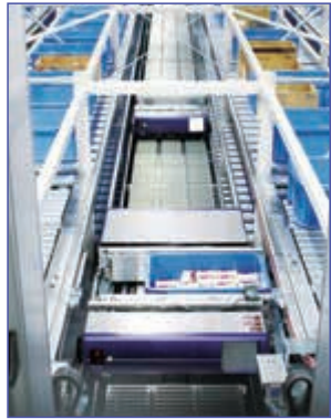
AS/RS* for picking operations Provides products in a timely manner to piece-picking robots
