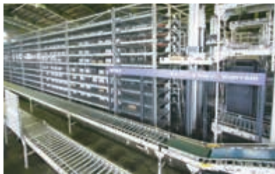
High-throughput mini load AS/RS – Shuttle Rack
