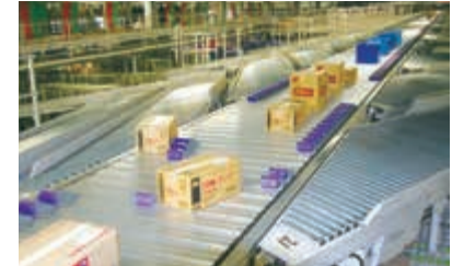
High-speed sorter – Surfing Sorter
