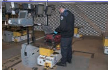
AGV-based mobile inspection table
