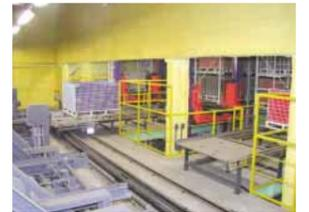
An AS/RS (right) and STV carrying fermentation pallets to inverting equipment for stirring
