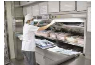
The VCR combines the function of storing irregularly shaped items of instruments with the ability to transport them between floors
