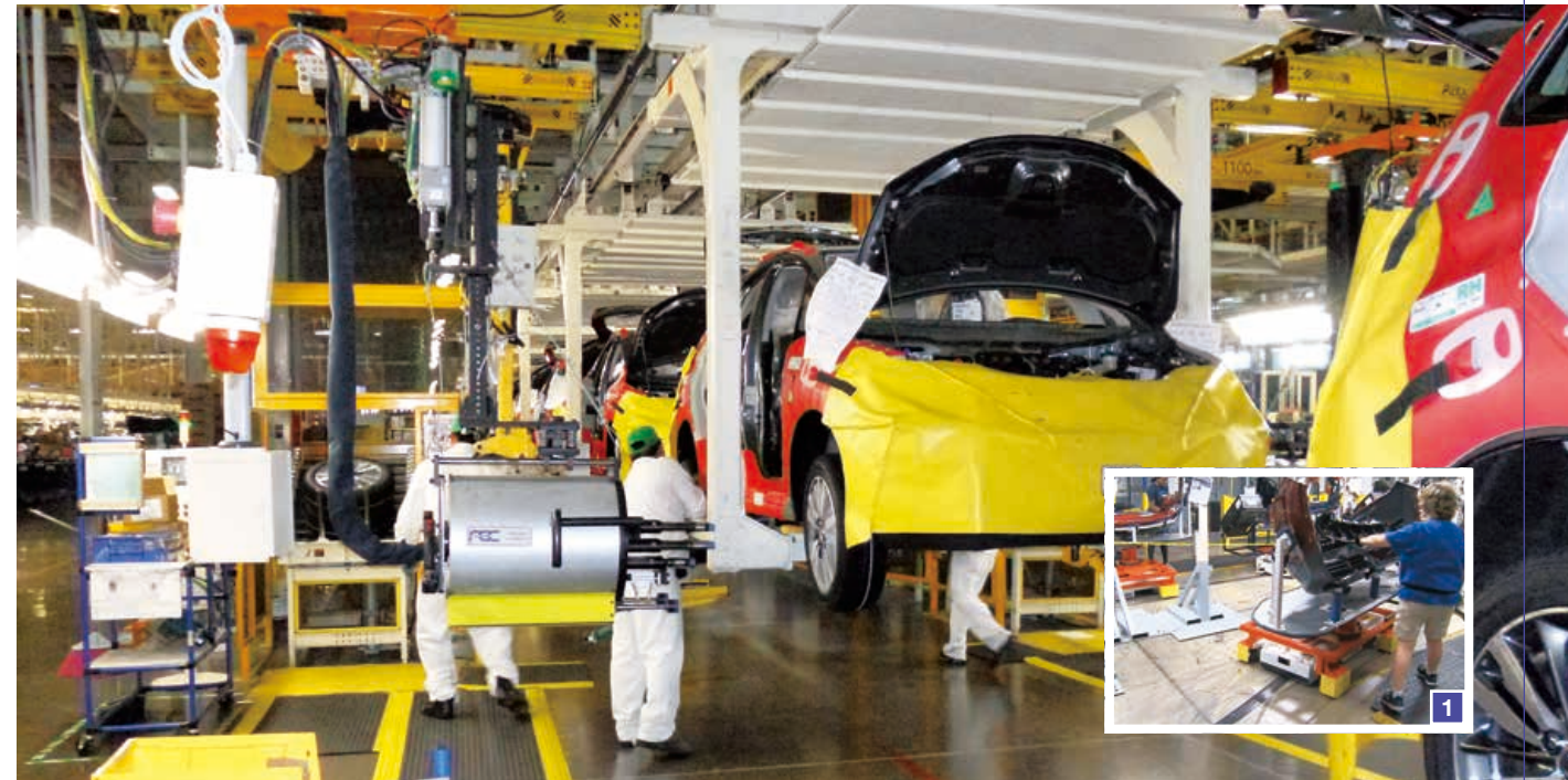
Overhead FDS chainless conveyor system on the assembly line of Honda de Mexico, S.A. de C.V.
