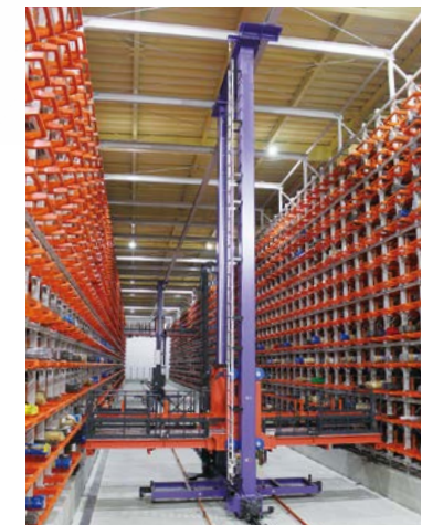
An automated warehouse system for long objects, one of the 2014 certified Eco-Products. By cutting its whole weight, the system saves energy in operation and reduces environmental impacts during production.
