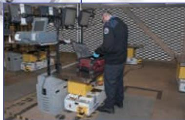
**AGV-based mobile inspection table**
