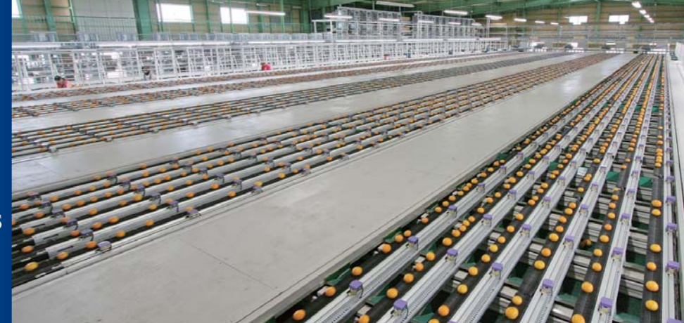
A fruit sorting Finger Domino Sorter used at Japan Agriculture Cooperatives (Kumamoto, Japan)
