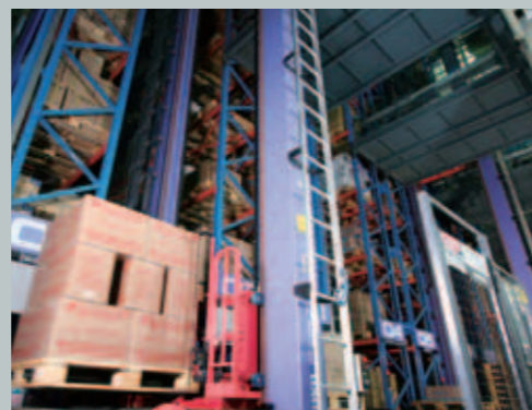
AS/RS installed at a pharmaceutical wholesaler
